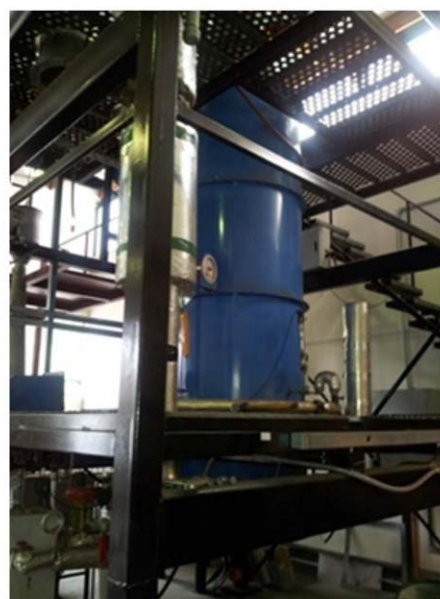
Figure 1. Flow diagram (a) and side view (b) of the bubbling fluidized bed system used for cogasification experiments in this study.
